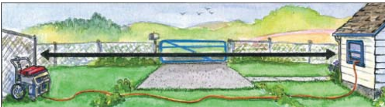
Figure 3-6: Use portable generators OUTSIDE and far away from the building.
