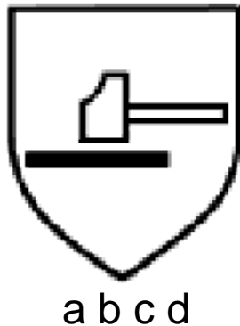
Pictogram employed to indicate glove performance against mechanical risks, as based on European regulation [AFNOR, 2004]
