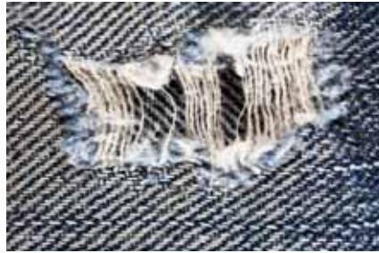
Textile that is threadbare due to abrasion
