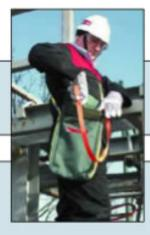
This shows the 'over the shoulder' style kit bag and 1 metre web lanyard in use. One end of the lanyard is clipped to the tool in use (in this case, a spanner). Kit bag with loops to attach to users harness is an alternative to this style and also exists.
