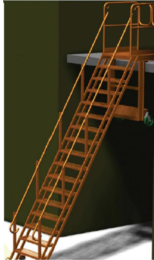
The portable stairs on the right are able to be reused on several projects while allowing the workers a safer angle for ascent and descent compared to the gang-ladder on the left.
