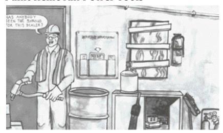
Lead paint is removed with power tools equipped with dust collectors prior to other lead-emitting activities. Small lead particles are collected by a HEPA vacuum system as they are released by the tools.
