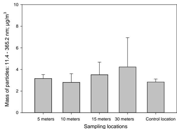
Figure 5. Mass concentration of total particles of 11.4 – 365.2 nm size range during wooden building frameworks construction.
