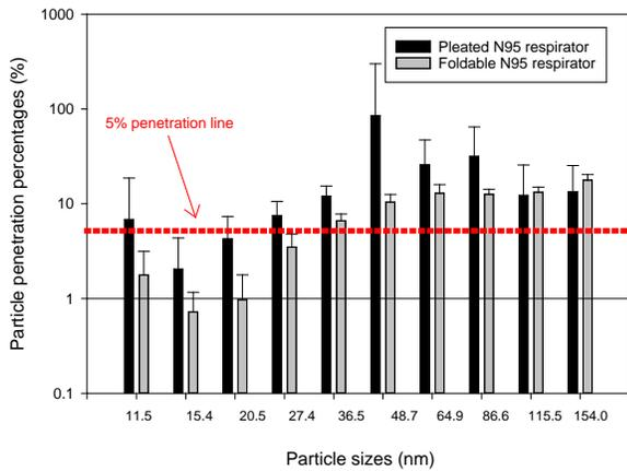
Figure 10. Penetration percentages of particles of 11.4 – 154.0 nm size range in isopropanol treated N95 masks during wooden building frameworks construction.
