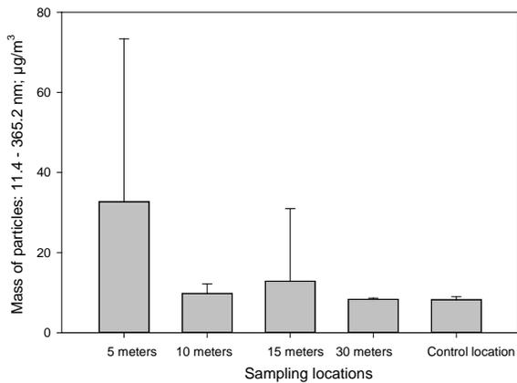
Figure 4. Mass concentration of total particles of 11.4 – 365.2 nm size range at concrete blasting and grinding site.
