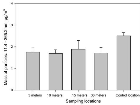
Figure 6. Mass concentration of total particles of 11.4 – 365.2 nm size range during soil moving at a large construction site.
