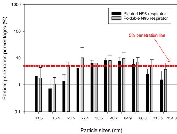
Figure 8. Penetration percentages of particles of 11.4 – 154.0 nm size range during wooden building frameworks construction.
