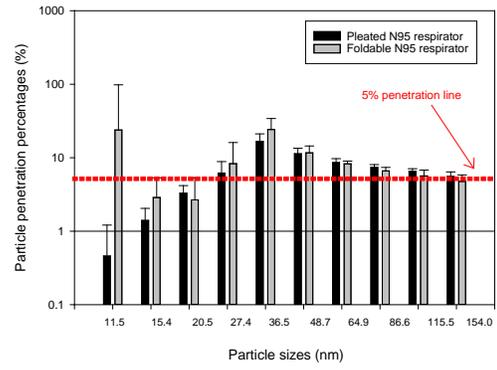
Figure 7. Penetration percentages of particles of 11.4 – 154.0 nm size range during concrete blasting and grinding.
