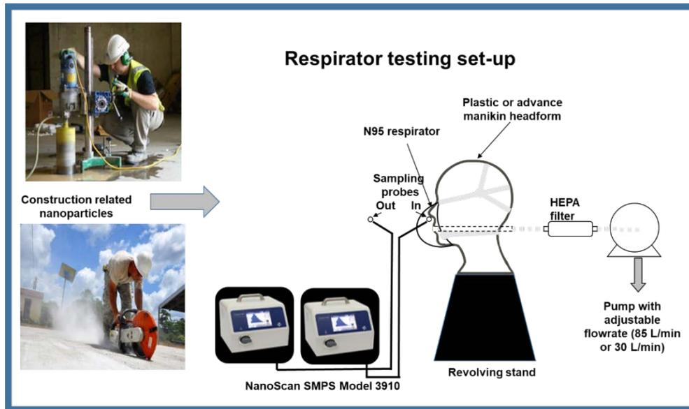
Figure 2. Schematic of the nanoparticle sampling system for assessing protection factors offered by N-series respirators in construction jobsites.
