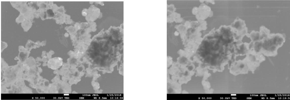
Figure 12. Scanning transmission electron micrographs of nanoparticles and agglomerates collected by the Sioutas impactor at construction sites.
