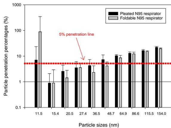
Figure 11. Penetration percentages of particles of 11.4 – 154.0 nm size range in isopropanol treated N95 masks during soil moving in a large construction site.
