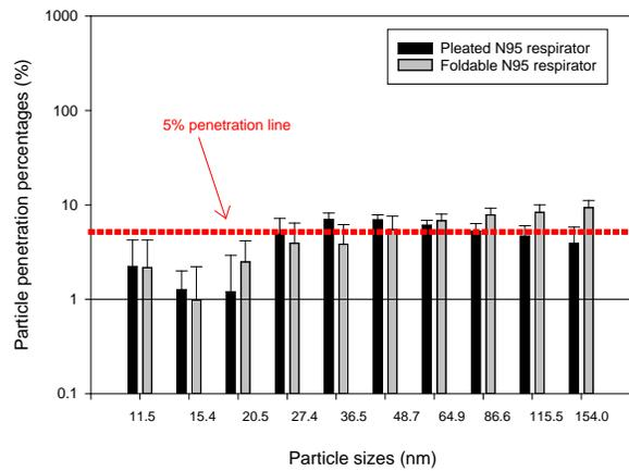
Figure 9. Penetration percentages of particles of 11.4 – 154.0 nm size range during soil moving by bulldozers in a large construction site.
