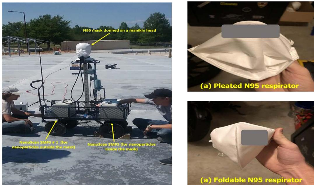
Figure 3. Manikin based N95 respirator evaluation system and respirators used in field experiments.
