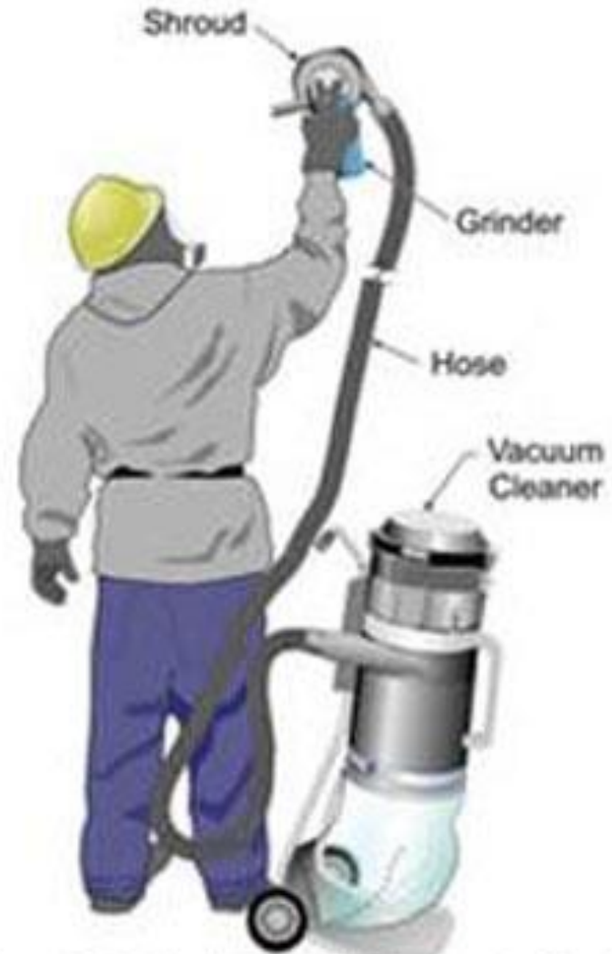
Figure 1. Grinder in use with the control in place.
