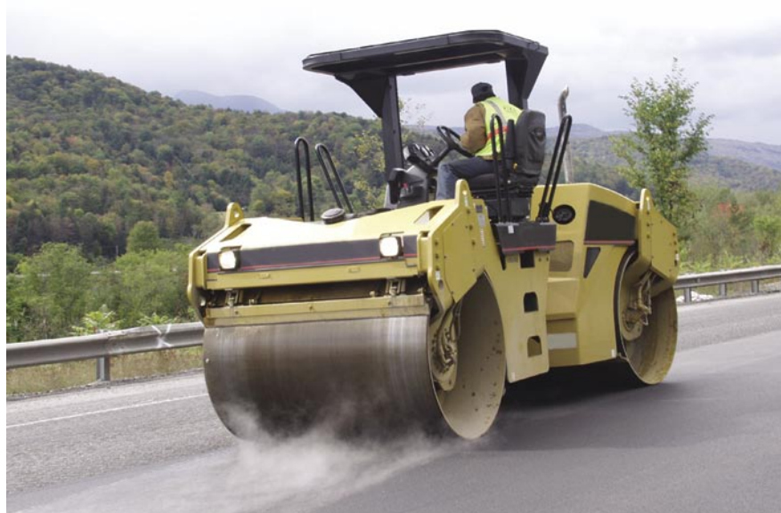
Ride-on roller/compactor with ROPS and seat belt
