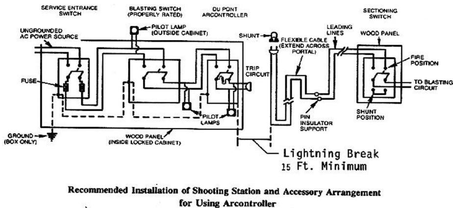
b. A grounded switch shall be installed between the blasting switch and the power circuit at a distance not less than 15 ft (4.5 m) from the blasting switch.
